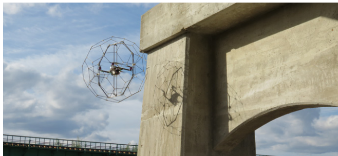
Checking bridge with spherical shell drone
