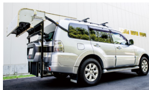
Capturing images of the road with stereo cameras and using artificial intelligence to automatically measure the extent of cracks
