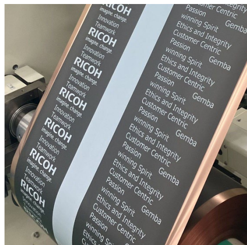
Fig. 19 Character printing on the electrode.
