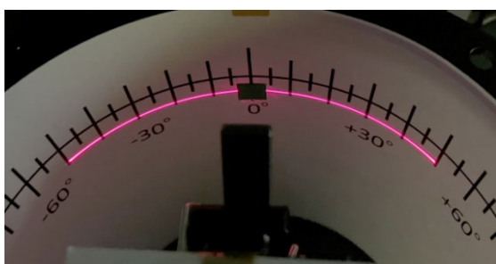
Fig. 8 Scanning line trajectory for optical scan angle of 98.8°.
