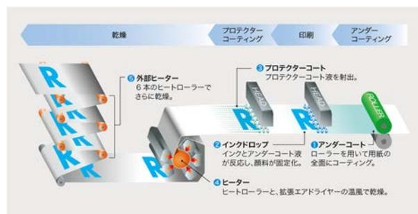
Fig. 3 Process of imaging on VC60000.
