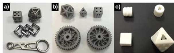
Fig. 12 Photographs of sintered parts examples; a) SUS316L, b) Titanium and c) Glass.
