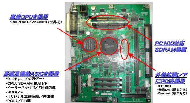
Fig.2 Millennium Architecture based IPSiO Color 8000 controller.
