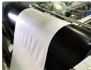
Cockling correction with heat rollers
