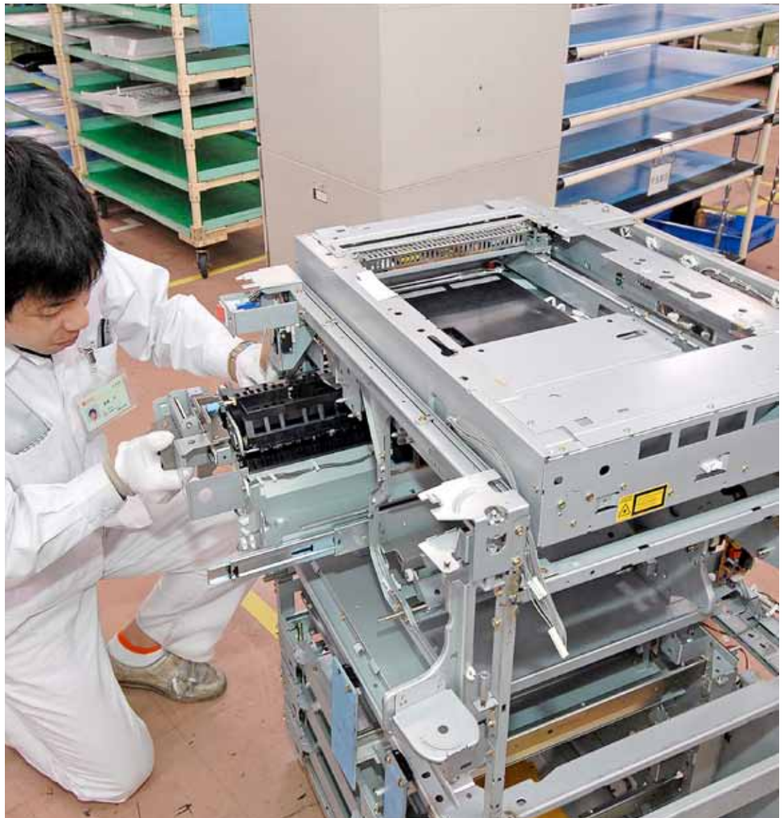
Used copiers are disassembled, have their parts cleaned, then reassembled.
