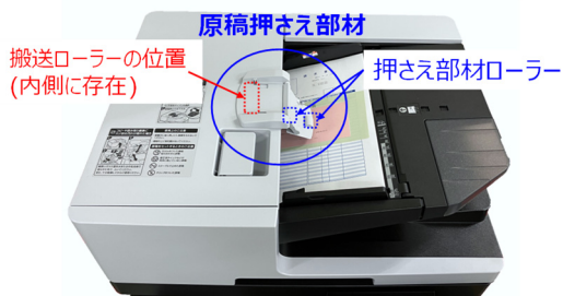
(a) External view photograph of the ADF with the component that holds down the document.
