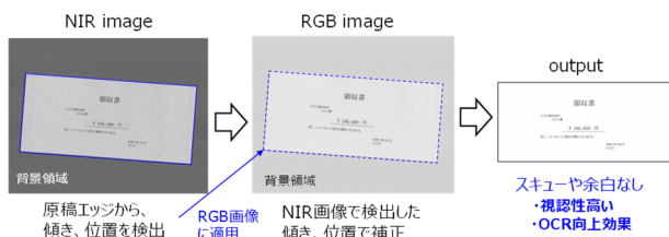
Fig. 13 Output image after skew correction and cropping.
