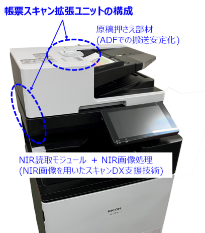
Fig. 2 External view photograph of the MFP with the document scanning extension unit installed.
