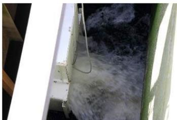
Fig. 11 Developed small scall hydroelectric power generation device in operation.
