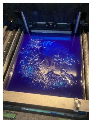
Fig. 1 Example of a failure due to collision between the object and the blade.
