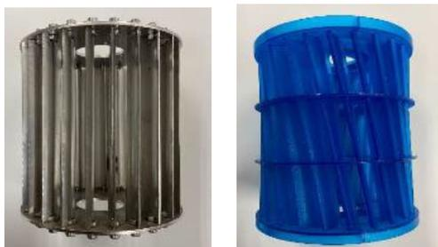
Fig. 8 Photo of metal water wheel and resin water wheel.
