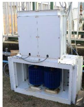
Fig. 10 Developed small scall hydroelectric power generation device.
