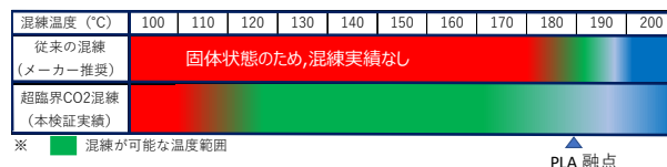
Fig. 8 Characteristics of kneading technology in the presence of scCO 2 .
