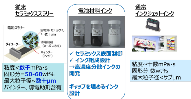
Fig. 4 Comparison of liquid properties among a conventional slurry, inkjet ink 16) and novel battery-material inks.
