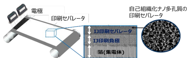
Fig. 8 Schematic view of separator printing and a cross section of the electrode with printed separator and a magnified view of internal structure of the printed separator.
