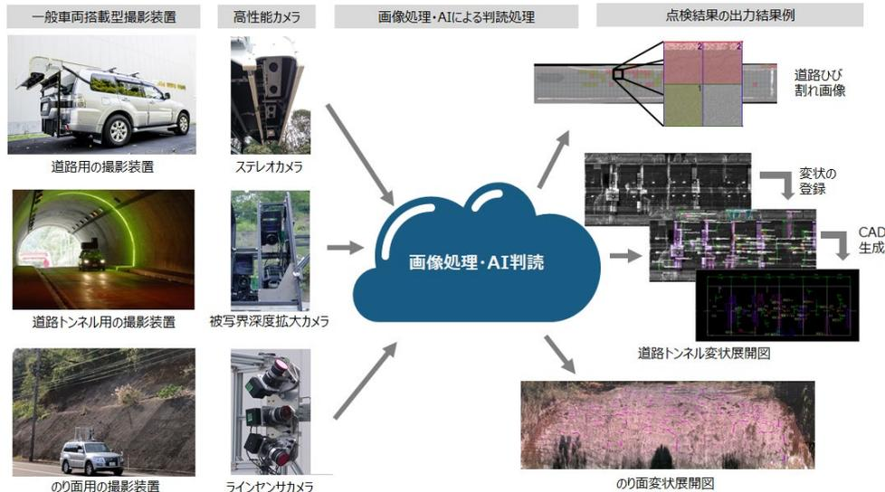
Fig. 16 Totalized inspection using unique camera and AI.
