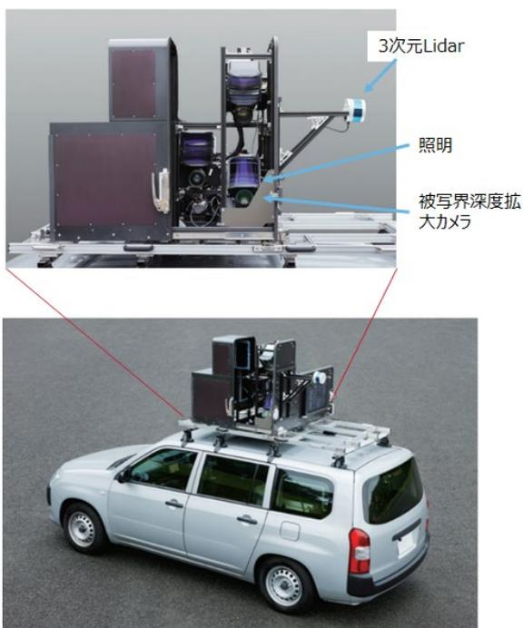
Fig. 6 Exterior of tunnel monitoring system by using line sensor camera with extended depth of field.
