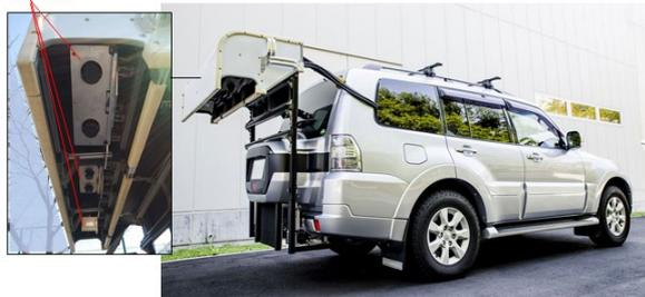
Fig. 1 Exterior of road surface monitoring system by using stereo cameras.
