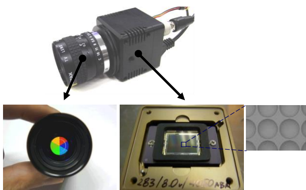
Fig. 5 Multi-spectrum Camera using Plenoptic System Left: Main Lens with multi-bands filters Right: Camera Sensor with MLA.
