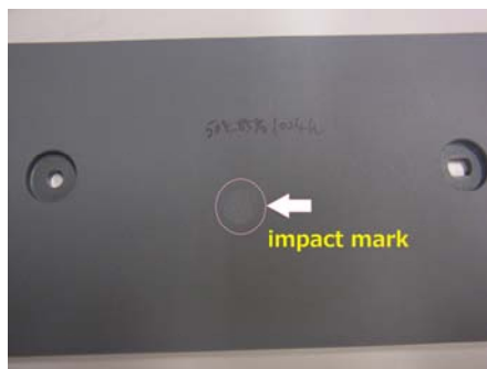
Fig.6 Picture of impact mark (standing time: 1000[hour]).
