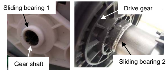
Fig.8 Photographs of worn-out gear bearings of the benchmark 2.
