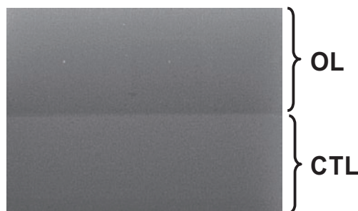
Fig.10 Cross sectional SEM view of organic photoreceptors.
