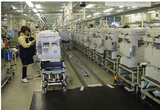
Fig.12 Push cart type production line.
