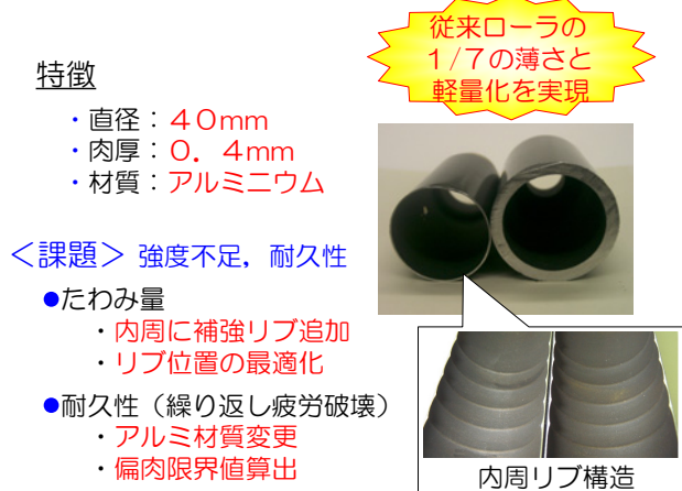
Fig.4 Ultra-thin shell type fusing roller.
