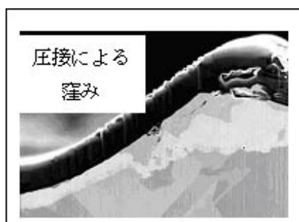
Fig.17 part of pure-Tin squeezed toward surface (white : IMC, grey : pure Tin).
