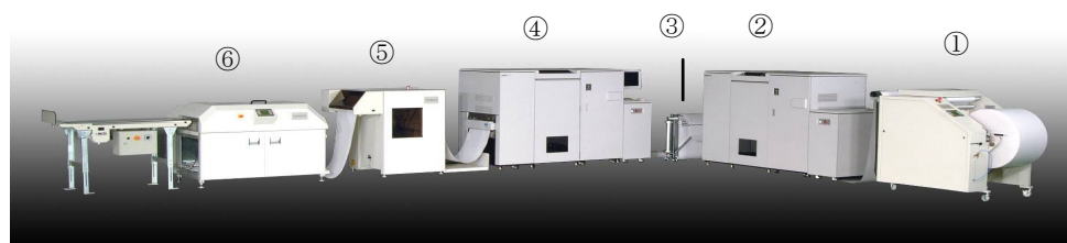
Fig.1 Tandem duplex printing system for roll paper.
