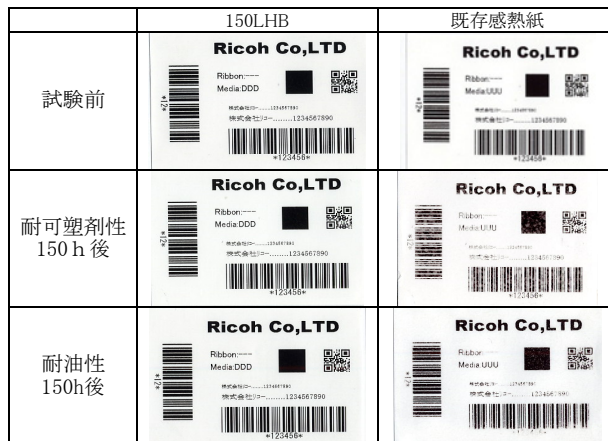
Fig.7 Sample of plasticizer and oil resistance.
