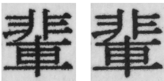
Fig.6 Plain paper Image comparison between. GELJET printer and Laser printer (RicohMF7070)
