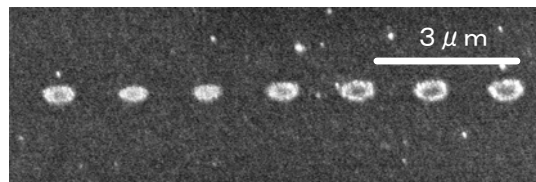
Fig.11 SEM image of the crystallized recording marks.
