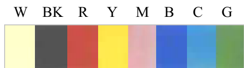
Fig.6 The sample was initialized to black color state by irradiating UV light. Then, respective position was irradiated by the lights with wavelength with 420nm+540nm+676nm(W), 676nm(R), 540nm+676nm(Y), 420nm+676nm (M), 420nm(B), 420nm+540nm(C) and 540nm(G).
