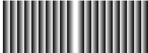
Fig.5 Projected patterns for the multi-region intensity ratio method. (a) A graded pattern whose light power for each region increases along projection angle. (b) A graded pattern whose light power for each region decreases along projection angle.
