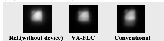
Fig.17 Projected pixel images on screen passing through the pixel-Shift Device.
