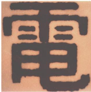
Fig.2 Printing samples printed by 600dpi TPH
