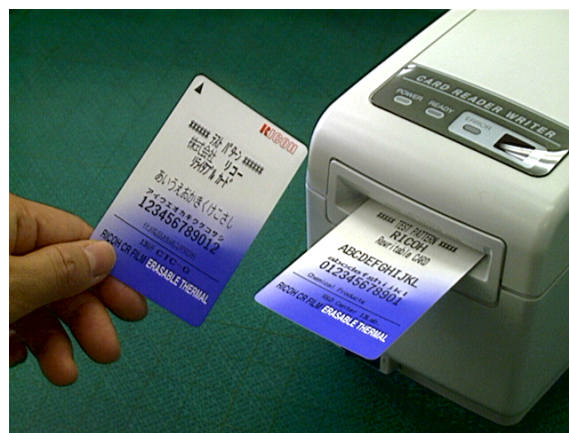
Fig.12 Rewriting black-colored images formed on the rewritable marking media using the new developers.
