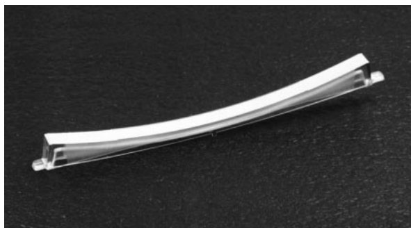
Fig.8 Picture of the aspherical f mirror
