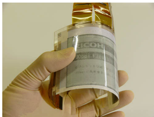
Fig. 1 Optical micrograph of a flexible EPD driven by a 160 ppi all-printed OTFT backplane.
