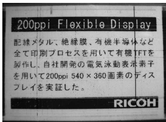
Fig. 8 Photograph of a 3.2 inch flexible EPD driven by a 200 ppi all-printed OTFT backplane (540 × 360 pixels).
