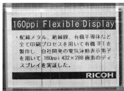
Fig. 4 A 160 ppi EPD driven by all-printed OTFT backplane on flexible substrates.
