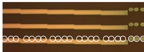
Fig. 5 Alignment margin of ink droplets ejected from IJ head onto the surface energy controlled polyimide film. White circles show impact positions of ink droplets
