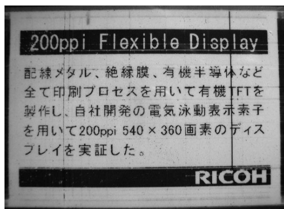
Fig. 11 Photograph of a 3.2 inch flexible EPD driven by a 200 ppi all-printed OTFT backplane (540 × 360 pixels)
