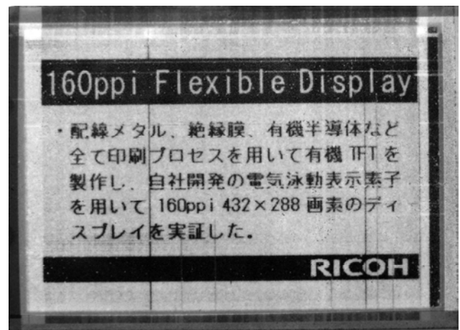
Fig.10 A 160 ppi EPD driven by all-printed OTFT backplane on flexible substrates.
