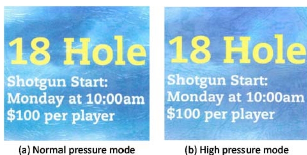
Fig. 10 Image samples printed out on the LEATHAC 66 (215 kg) with the elastic intermediate transfer belt.
