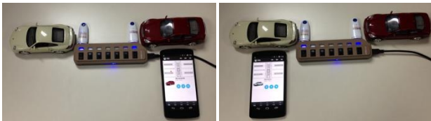
Fig. 4 "Smart MICE" mobile application automatically displays nearest exhibit's information (a BLE dongle is deployed for each exhibit).
