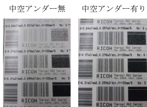
Fig. 12 Photographs of print with and without balloon particle.
