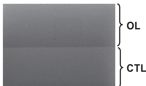
Fig.10 Cross sectional SEM view of organic photoreceptors.
